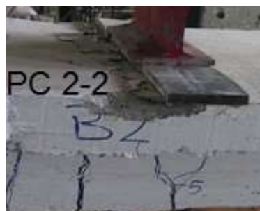
Fig.6: Crack pattern of girders (PC 2-1, PC 2-2, and PC 2-3 and PC 2-4 respectively)
