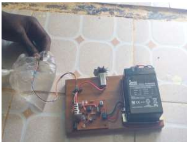
Plate 3: Testing the response of the solar powered fan at low temperature
