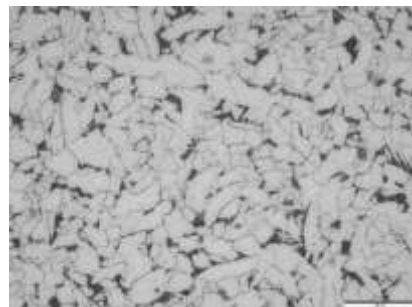
Fig.16: Microstructure of re-heat refined zone in weld deposit due to P-GTAW + HF dressing
