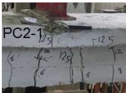
Fig.6: Crack pattern of girders (PC 2-1, PC 2-2, and PC 2-3 and PC 2-4 respectively)
