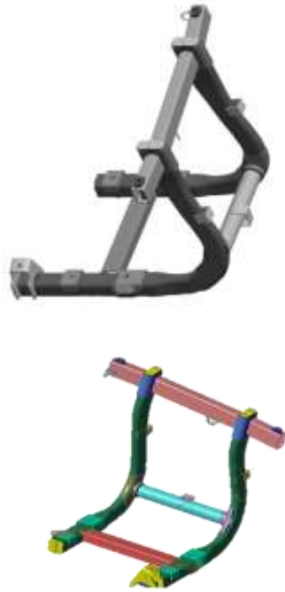
Fig.9: Modified design of engine supporting bracket for 3-D Model
