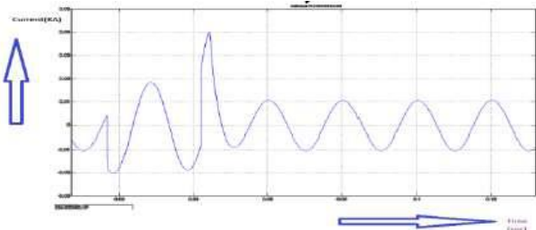
Fig.10: Current waveforms at PCC without FD-STATCOM
