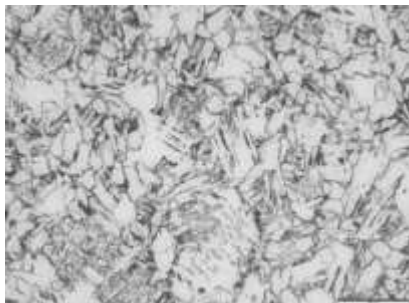
Fig.12: Microstructure of dressed weld deposit by P-GTAW
