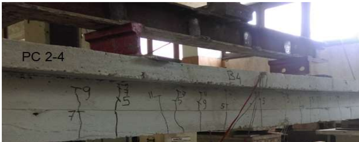
Fig.6: Crack pattern of girders (PC 2-1, PC 2-2, and PC 2-3 and PC 2-4 respectively)
