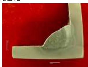
Fig.1: Typical macrograph of Undressed weldment
