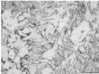
Fig.12: Microstructure of dressed weld deposit by P-GTAW
