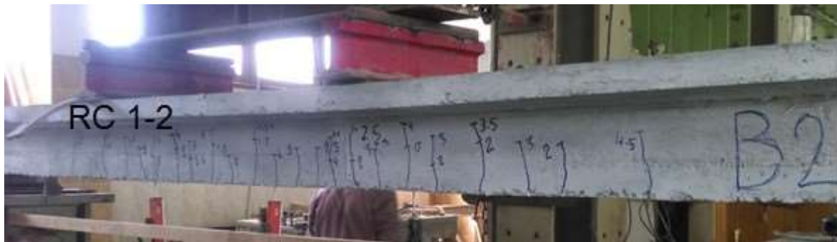
Fig.5: Crack pattern of girders RC (1-1) and RC (1-2) respectively
